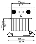
The compact STVS CX5030T is a next-generation dual-energy X-ray system engineered for seamless inspection of hand-held baggage, parcels, and briefcases. Weighing less than 465 pounds with tunnel dimensions of 21" wide by 13.1" high, CX5030T can be easily transported and rapidly deployed to meet evolving security needs.
